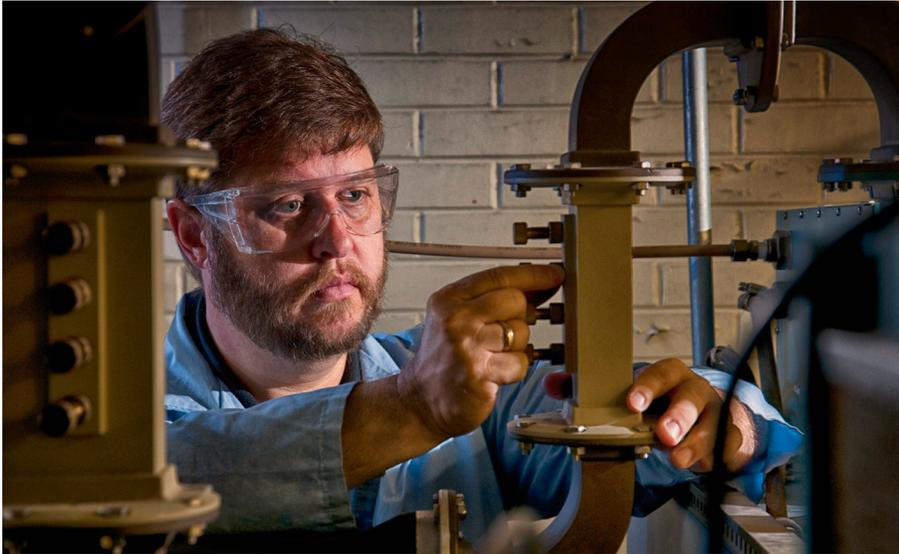
For more than two decades Y-12 has been developing microwave metal and ceramic processing technologies related to melting, casting, heat treating, sintering and bonding. Recent developments include vast improvements in ceramic systems that provide ways to heat materials not readily amenable to microwave processing.
